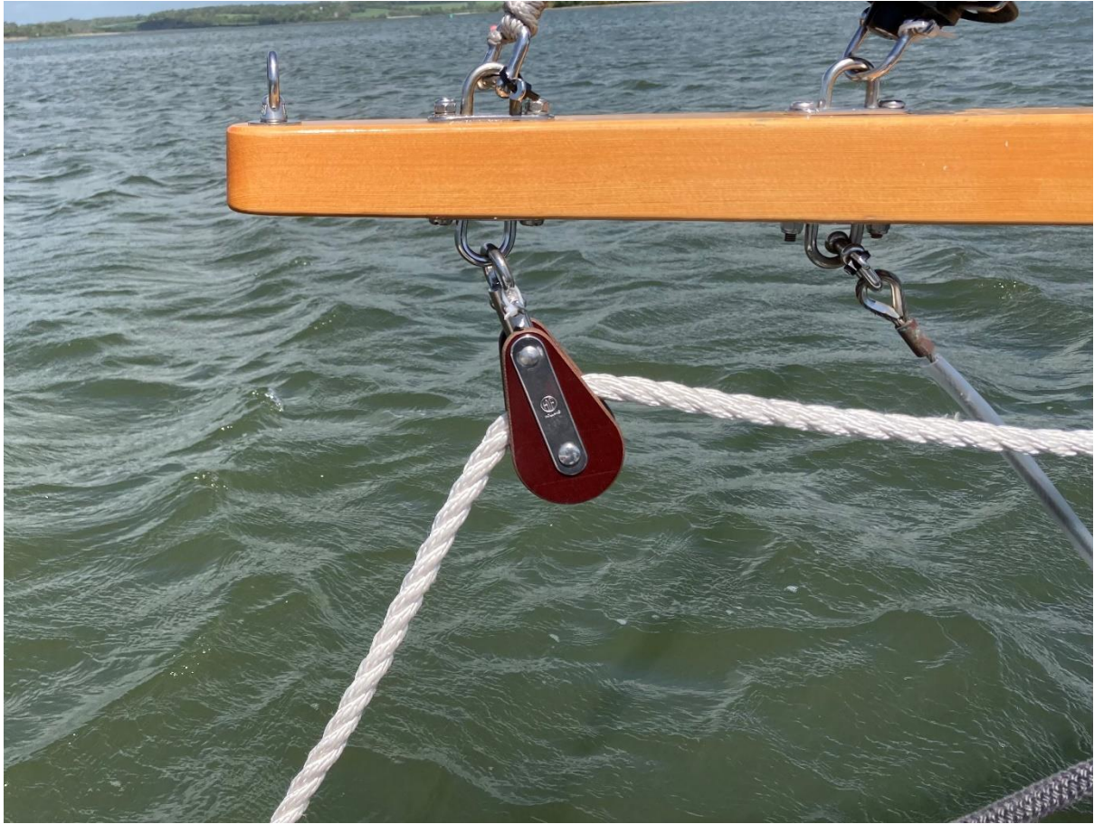
PHOTO 1 (the position of the swivel type pulley block)
