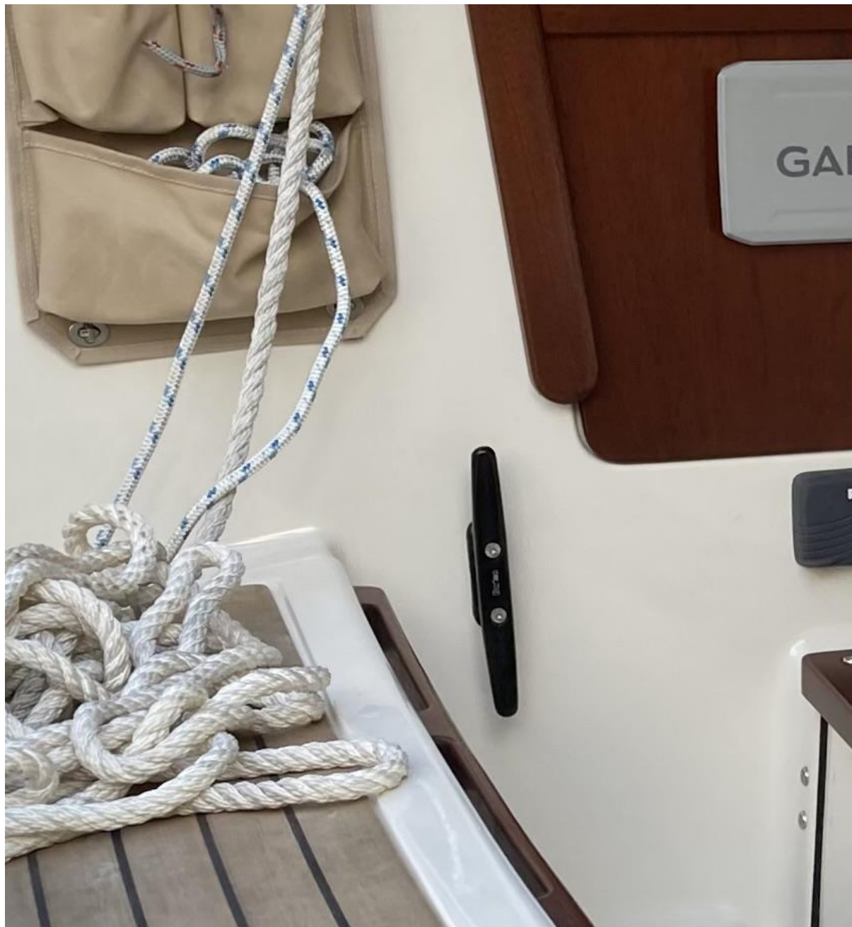
PHOTO 3 (the strong anchor cleat mounted on the cabin bulkhead)
