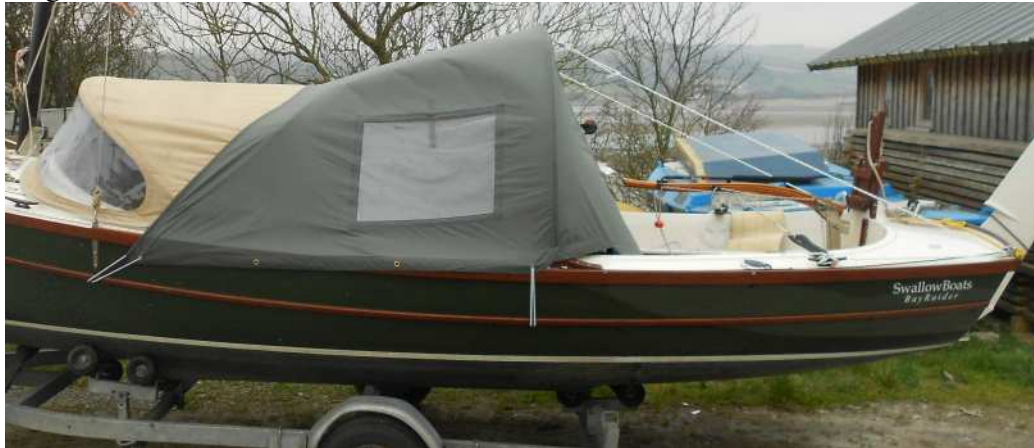
Above: Note the guy ropes are lead back through the aft fairleads to improve lead angle
