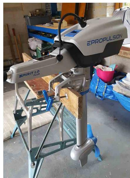
As supplied, the prop shaft is rotated 180 degrees from straight ahead and the tiller arm folded right down parallel to the shaft, which is the compact form for carrying and also how it fits into the carry (guitar) bag I'd also ordered. It goes nicely onto the back seat of a car and also fits easily into a BRe cockpit locker.
