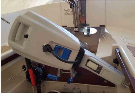
and also means that the back of the battery is well down and out of the way of any rigging, tiller ropes etc. This position also gives easy presentation of the control lever for raising and lowering the motor.
