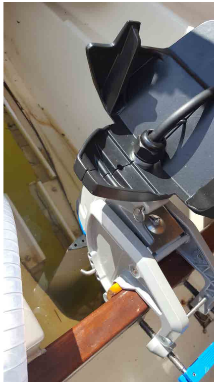
Above: Showing the small wedge in position, the prop angle pin in its second position, and the snug fit of the prop shaft in the engine well when rotated 90 degrees.
