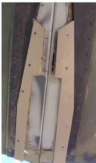
ing than garden machinery. I put my hand through the lamellae and immediately cut my fingers. Replacing the lamellae with a cover plate is much discussed on the forum but most solutions go the 'Full Monty', removing the whole lot. I had another idea - to create a keyhole shaped cut-out and hatch cover just big enough for raising and lowering the motor.
