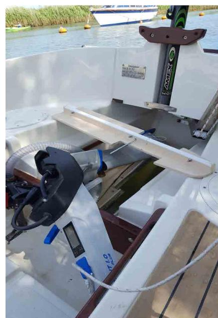
Secondly the cover plate is easy to hold by its narrow section and locates easily. Thirdly you can use the cover plate as a poker to prod the propeller into a vertical position to come up through the aperture if needed. Finally the centre part is narrow enough to easily arrange a locating pin.
